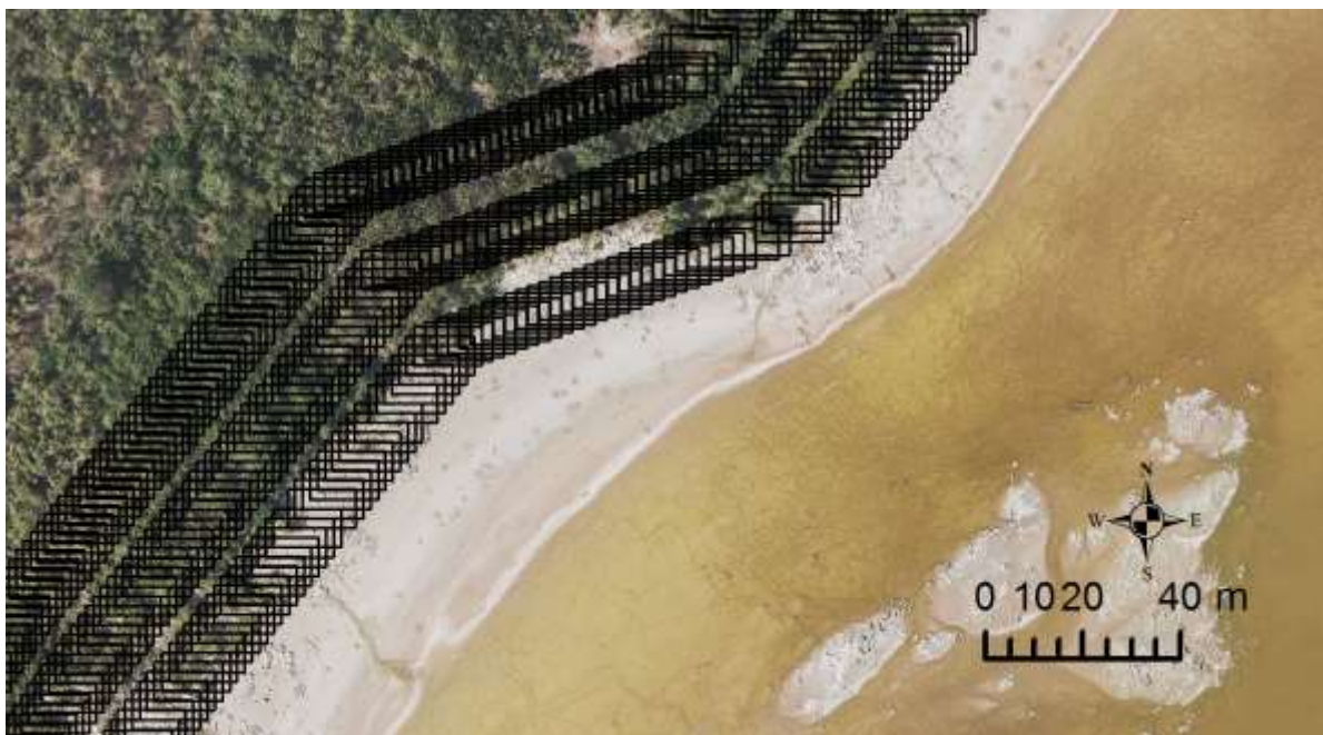
Figure 2.3 Rectangular boxes displaying the cameras field of view on each flight line, on ArcGIS.
